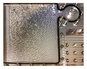
The simulation-enabled process generated highperforming designs that resemble natural fluid reactant-distributing structures, such as leaves, lungs, and blood vessels.
