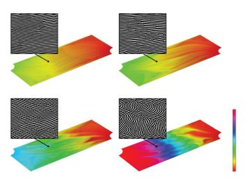
Applying this process resulted in four distinctive microchannel designs, all of which outperform baseline conventional designs across key reactionfluid performance metrics.
