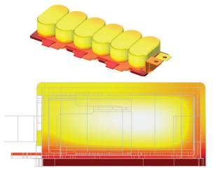
Modeling DC link capacitors has enabled the team to identify potential "hot spots" early in the development process, making it easier to avoid the failure that can result from too-high heat.
