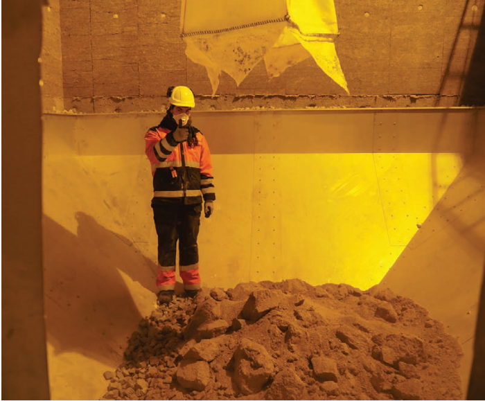
FIGURE 3 Markku Ylönen with a representative sample of Polar Night Energy’s dirt-cheap heat storage medium.
