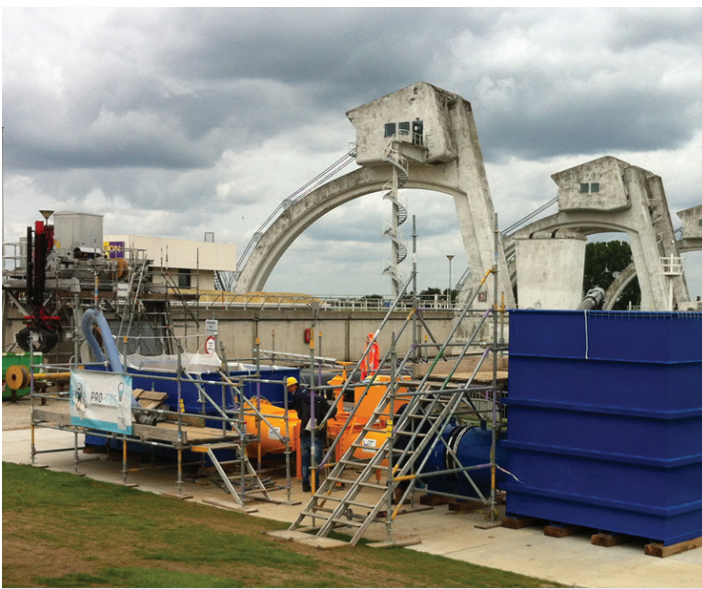
FIGURE 7 The Water2Energy water turbine prototype, about to undergo live testing.
