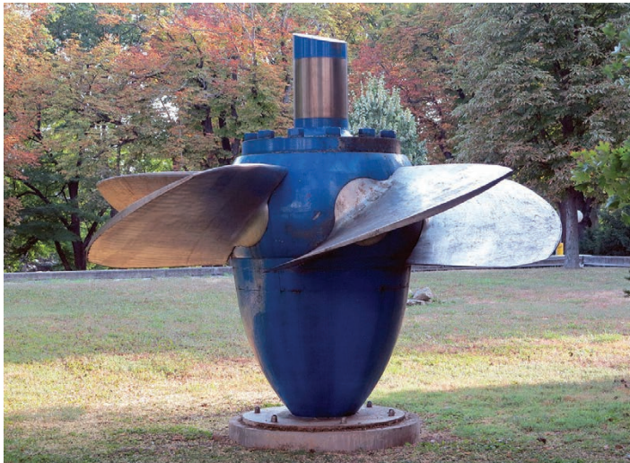
FIGURE 2 An example of a Kaplan turbine rotor. Image by Reinraum, CCO, via Wikimedia Commons.
