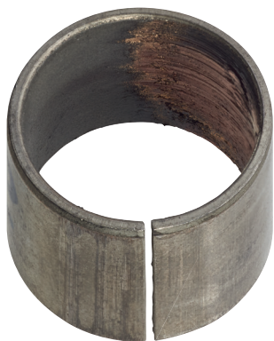
Worn sliding layer (top) and corrosion (bottom) of PTFE-lined metal backed bearings
