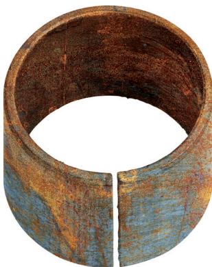
Worn sliding layer (top) and corrosion (bottom) of PTFE-lined metal backed bearings
