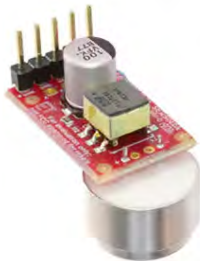
Figure 8: The PGA460PSM-EVM evaluation module is based on the PGA460 and simplifies the exploration of ultrasonic system operation using the PUI Audio UTR-1440K-TT-R 40 kHz ultrasonic transceiver. (Image source: Texas Instruments )
