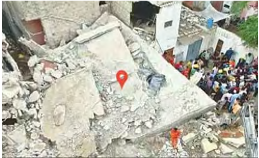
Figure 4: A drone's-eye view of a collapsed building is an important first step a drone would take with a conventional camera. Then, with the use of a thermal imaging camera, it could sense the body heat of those trapped in the rubble. (Image source: IEEE 4 )
