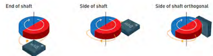
Figure 2: Designers can choose a magnet-to-sensor position based on design considerations such as the required level of immunity to external field disturbance and air gap tolerance. (Image source: Monolithic Power Systems)
