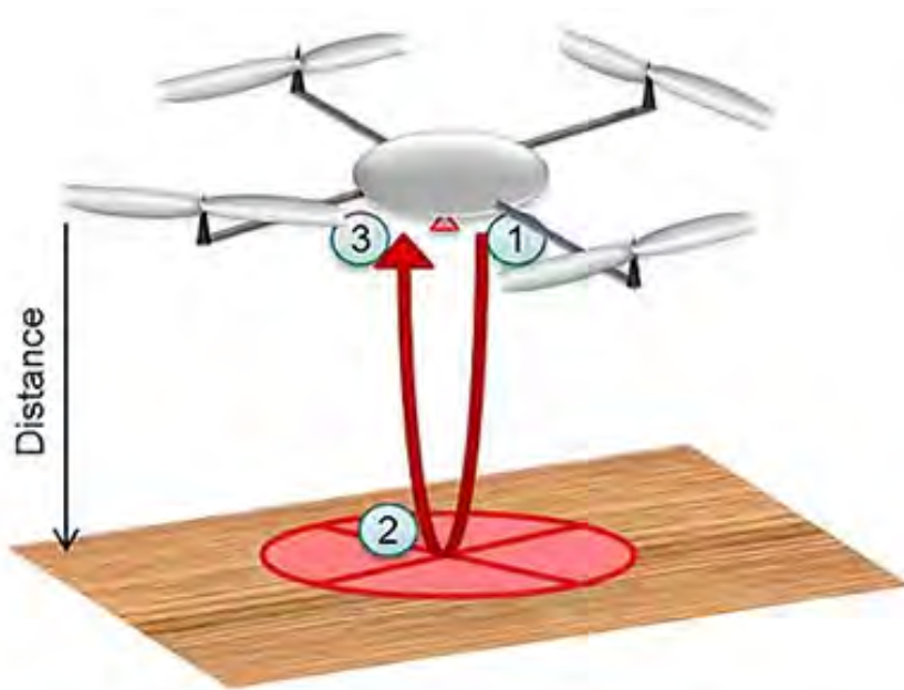
Figure 2: Designers will need to understand the concepts of ToF during a drone landing, hovering, or wireless charging. (Image source: Texas Instruments)
