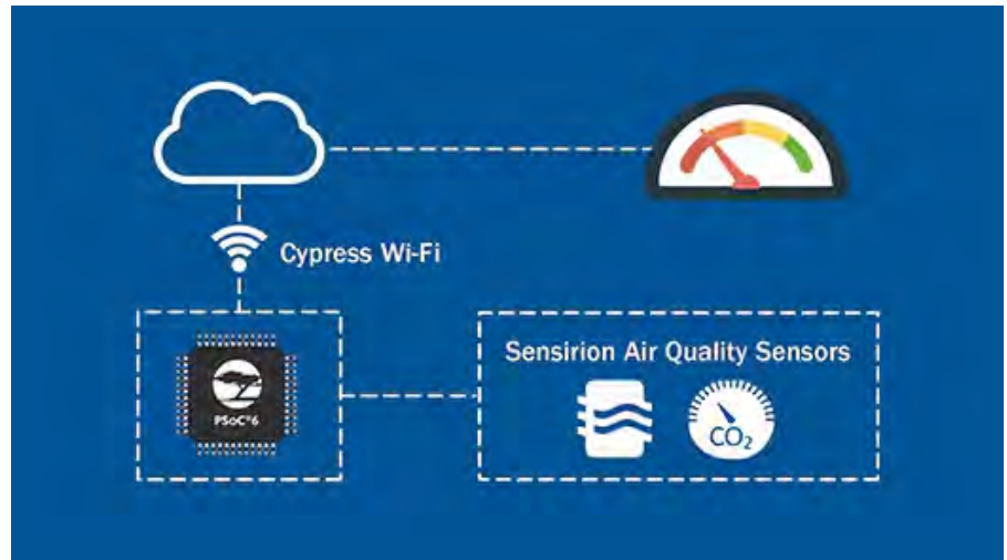
Figure 4: This dev kit from Sensirion and Infineon can implement secure boot and secure firmware updates. (Image source: DigiKey)
